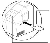
**2.** Insert one Pre-Saturated Cleaning Card (provided) through slot on the side of the Card Cartridge.
